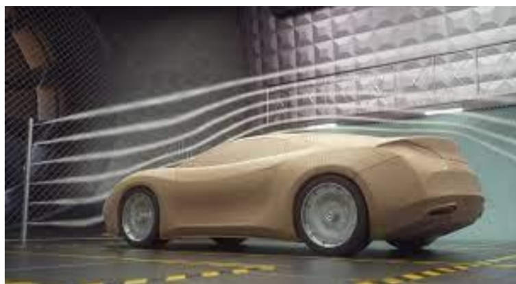
2-rasm. Avtomobilning masshtablashtirilgan modellarining aerodinamik sinovdan o'tkazish
